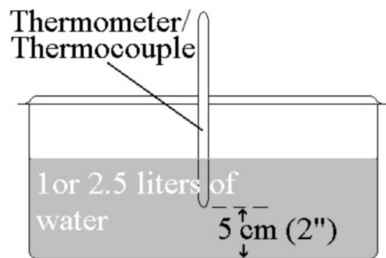
The lower tip of the thermometer or thermocouple shall be mounted and fixed 5 cm (2 inches) above the bottom of the pot.
