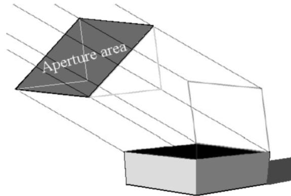
The above picture shows the aperture area of a box cooker.
